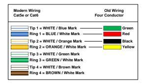
"Tip" and "Ring" are common terms in the telephone service industry referring to the two wires or sides of an ordinary telephone line. Tip is the ground side (positive) and Ring is the battery (negative) side of a phone circuit. The ground side is common with the central office of the telephone company (telco); the battery side carries -48 volts of DC voltage when in an "idle" or "on hook" state.
